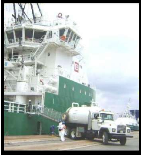
Sludge Evacuation from Bourbon Diamond Vessel
