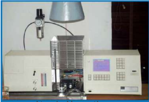
Atomic Absorption Spectrophotometer (AAS)
