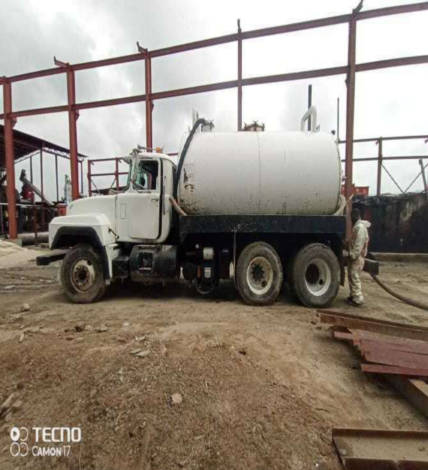
TMCH VACUUM TRUCK EVACUATING WASTE SLUDGE FROM SHELL BODO PROJECT SITE FOR ONWARD DELIVERY TO THE TREATMENT FACILITY
